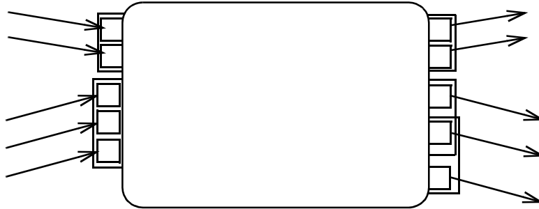
Figure 12.117 - Alternative input/outputs using parameter sets notation
