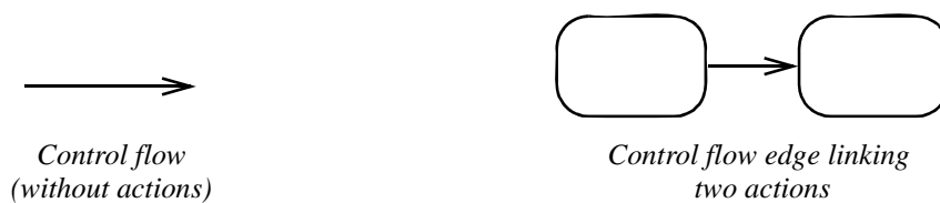
Figure 12.70 - Control flow notation
